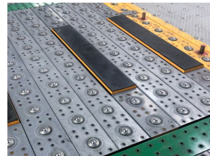
Pneumatic stops prevent the ULD from moving for safer loading processes
