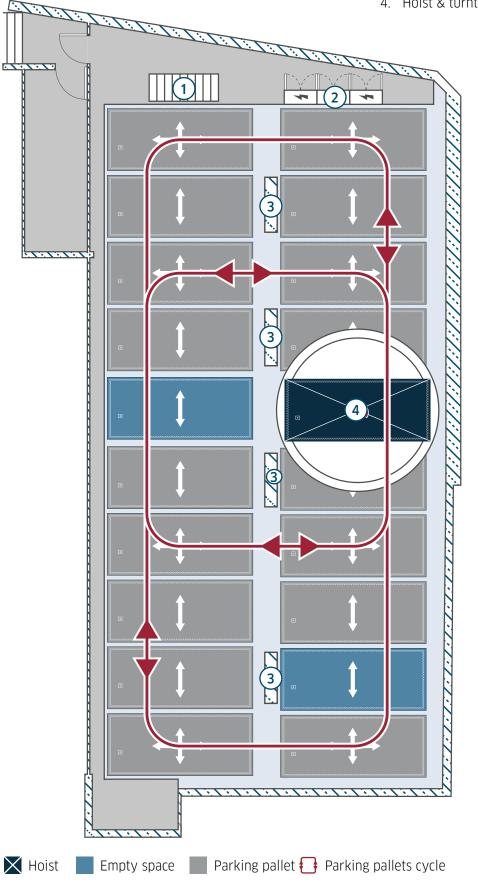
Fig. 21: Complete overview of the RESPACE<sup>®</sup> system with accesses, switch cabinets, and maintenance openings.
