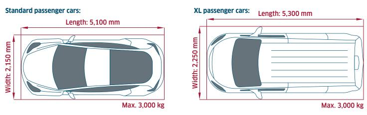
Fig. 3: Vehicle dimensions for the RESPACE<sup>®</sup> parking system.
