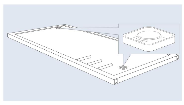
Fig. 19: RESPACE<sup>®</sup> pallet with EV-charging sockets.
