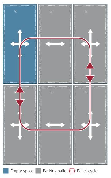
Fig. 6: Simple RESPACE<sup>®</sup> parking system with four parking spaces and integrated hoist.
