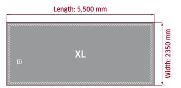
Fig. 5: Pallet sizes in the RESPACE<sup>®</sup> system.
