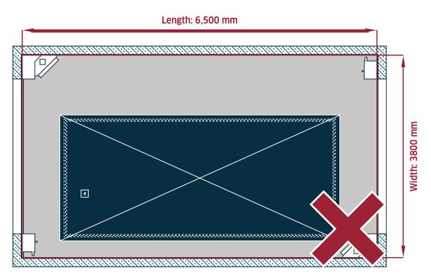
Fig. 17: Incorrect placement of the hoist in the cabin as the pallet is no longer aligned with the cabin gate.
