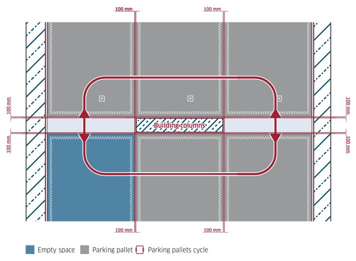
Fig. 8: Parking system with five parking spaces (standard pallets) and integrated building support.
