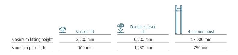
All standard hoists are devised so that models with longitudinal, traverse or bidirectional conveyors or models with rotary table function can be provided. Scissor and double scissor lifts will be delivered with a self-supporting steel structure. For a 4-column hoist, this same steel structure must also be attached to the shaft in some places. An opening for the pallet size plus 100mm circumferential space must be provided for the ceiling opening in the transfer cabinet in the area of the hoist.
