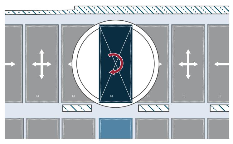
Fig. 12: Integrated turntable
