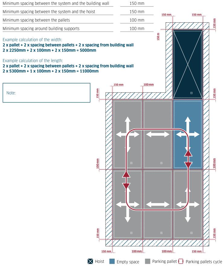
Fig. 7: Parking system with five parking spaces (standard pallets) without building supports.
