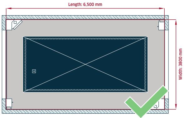
Fig. 16: Correct placement of the hoist in the cabin.
